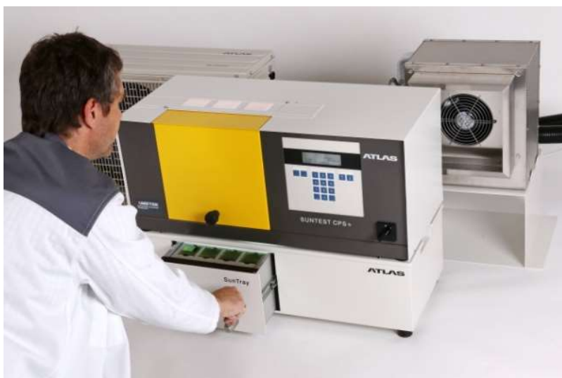
Picture 2: In vitro UVA test setup with SUNTEST CPS+, SunCool and SunTray accessories
